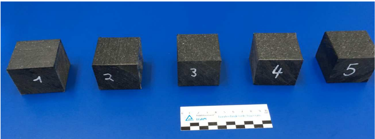
Fig. 1: Plate Type 1: Dimensions: 50 mm x 50 mm x 40 mm, test specimen 1 to 5
