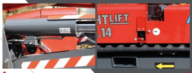
Outrigger block valves doubled for safety, also protected from accidental impact. Auxiliary connector for external devices, telematics and fleet tracking.
