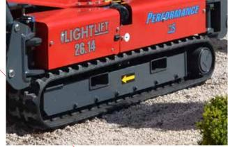
Large forklift pockets to allow easy lifting with forklift or tele-handler to load, unload and transport the machine.
