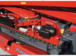
110V-220V electric motor with improved torque.
