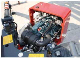
New Kubota Diesel D902 3 cylinder water cooled engine, meets the Tier 4 standards, with 40 litres capacity tank for an increased range.
