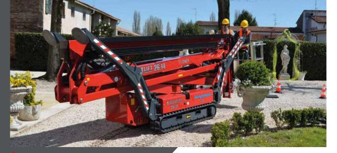
Lengthened undercarriage for greater stability, improved angle of attack (22°) and lowering of ground pressure during translation, equipped with Auto2Speed technology for maximum speed or torque depending on the working conditions.
