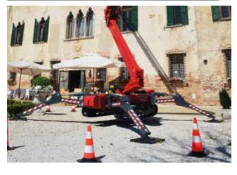
Assisted automatic stabilization on slopes, up to 16°. Allows a ground clearance of 700mm with machine completely stabilized, with slope control during destabilization.
