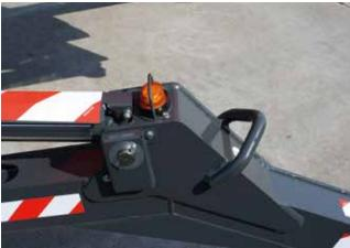
New low energy LED lamps on outriggers. Heavy Duty lifting hooks on outriggers for quick and easy positioning with crane.
