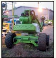
The **HR18** offers exceptional rough terrain performance due to its increased wheel size and ground clearance. Add to this a class leading working envelope and spacious 300kg capacity platform and the **HR18** stands out as one of the most robust and versatile work platforms available.
