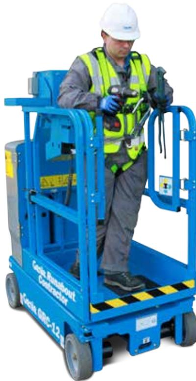
*Specifically designed to help an operator easily get in and out of the basket, with tools and jobsite materials.*
