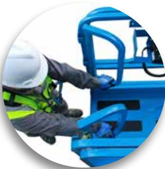
*The saloon doors allow for walk-in access to and from the basket when operators are wearing a tool belt.*
