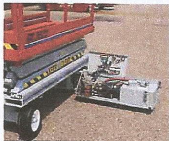
"Swing-out" drawers permit full access to all hydraulic and electric components for easy service and maintenance.
