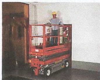
Narrow width allows SJII Model 3220 to pass through standard doorways and narrow aisles.
