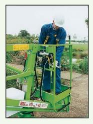
The Nifty 90 has a telescopic axle allowing it to pass thorugh a 0.75m (2ft 6in) opening and a harness point in the platform for operator safety when working.
