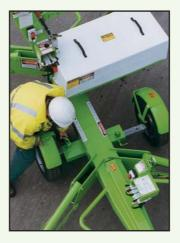
Retractable axles allow the Nifty 120 to pass through a 1.10m (3ft 6in) wide opening.
