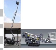
lift that can be made very narrow transport width. Suitable for narrow driveways and work on inclined surfaces. Good overhang sideways and up and over reach. The lift is run on either diesel or direct current. Each track is gray non- marking.
