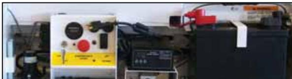
The HB-1030CE utilizes a highly efficient 24 vdc electrical system and includes an integrated battery charger with charge level indicator, descent and tilt alarms, palm button emergency stops, remote raise/lower station and key switch. Our open bay design provides direct access to all critical components. This innovative design feature reduces repair time, helping keep costs down.
