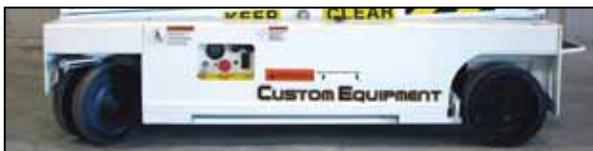
Non-marking tires, with a unique dual-wheel front steering system eliminates floor scuffing and carpet buckling, helping prevent damage to sensitive and/or decorative flooring materials. The HB-1030CE's design includes pothole protection and meets or exceeds applicable OSHA, EN280, and ANSI A92.6-1999 safety standards.
