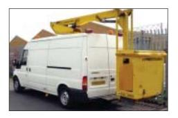
The **Gardner Denver DA range** of work platforms provide simple, reliable and low cost performance giving zero tail swing with working heights from 10.5m-14.0m. All are suitable for mounting on van or chassis cab vehicles.
