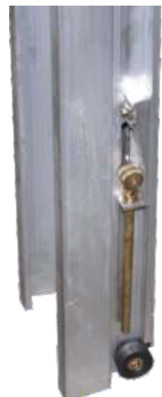
Safety brakes fitted on both sides
