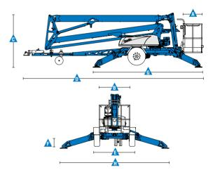
\* The metric equivalent of working height adds 2 m to platform height.
