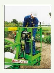
The **Nifty 90** has a telescopic axle allowing it to pass through a 0.90m (2ft 11in) opening and a harness point in the platform for operator safety when working.
