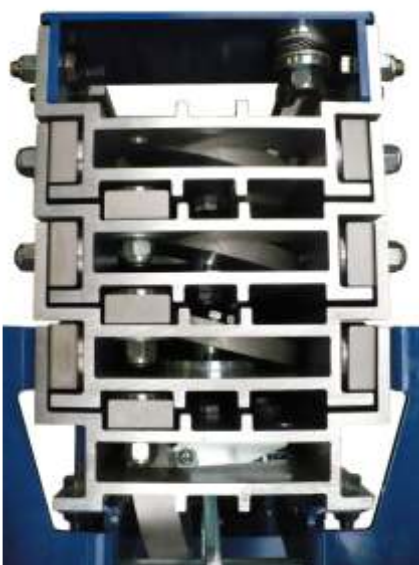
Mast system with special profiles and bearings.
