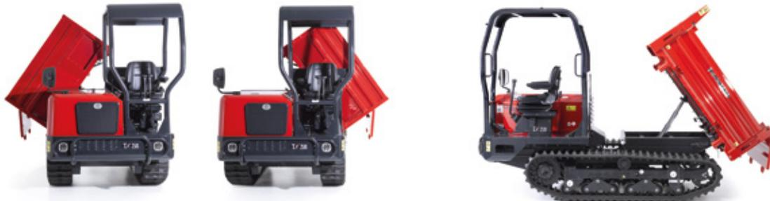
Triple flange rollers are designed to make TX2500 drive safe on slopes and rough terrain, as they ensure stability and reduce the risk of untracking. The short pitch offers smooth drive for optimal comfort at high speed.
