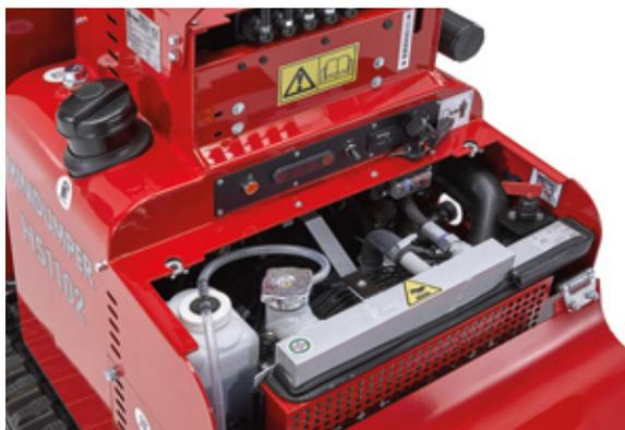
▲ The new housing is designed to allow a simple inspection/routine maintenance thanks to the improved engine access.
