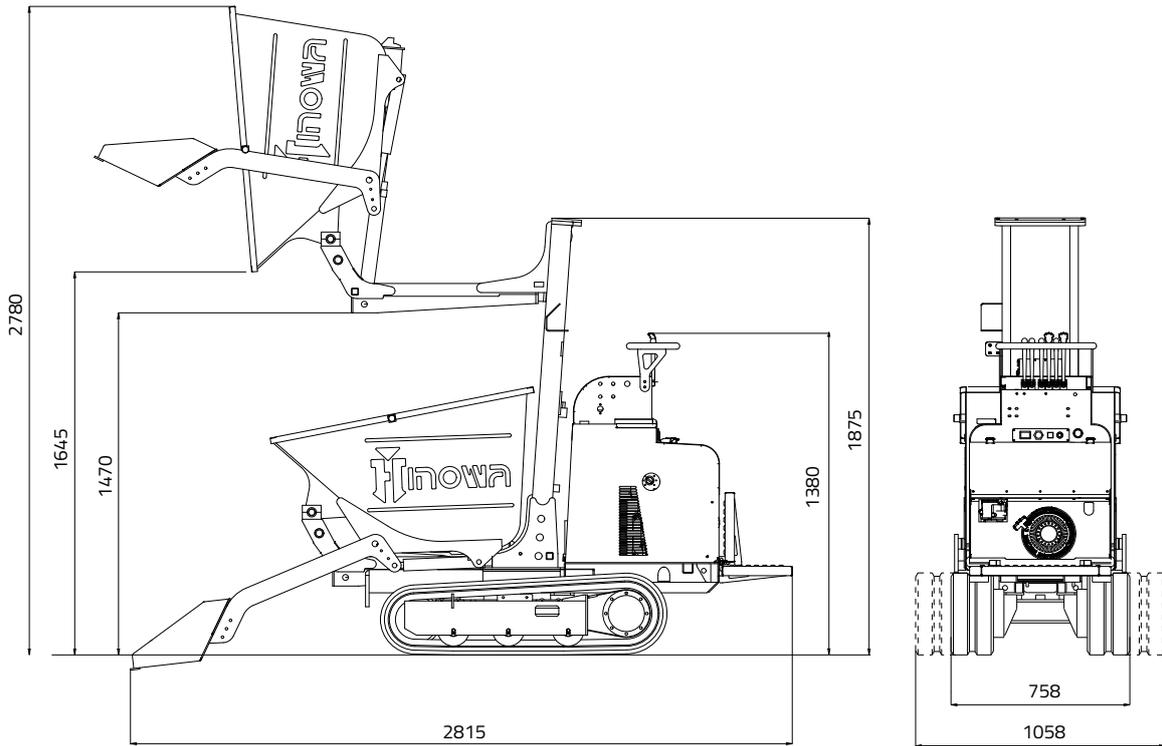
The unique self-loading, high dumping system with vertical guides
