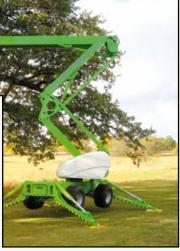
The extra manoeuvrability available from the 4 wheel steer option coupled with the special "Turf Tyres" make the **SD210** ideal for working on sensitive surfaces such as grass.
