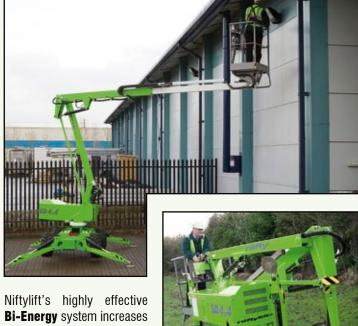
**Bi-Energy** system increases flexibility and maximises utilisation allowing the **SD120T** to operate for longer and in a wider range of environments.
